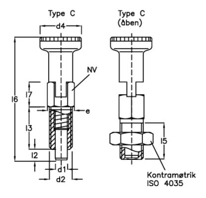
d1 = 8 I7 = 13.5 d2 = M12 NV = 12 d4 = 21 Spring pressure N bottom = 22 e = 13.8 Spring pressure N top = 6 I2 = 8
